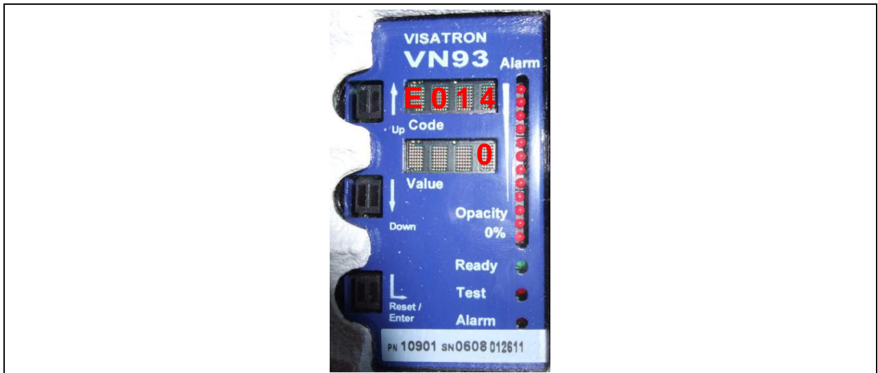
Figure 40: Device not ready, example of 'Negative pressure too low'
