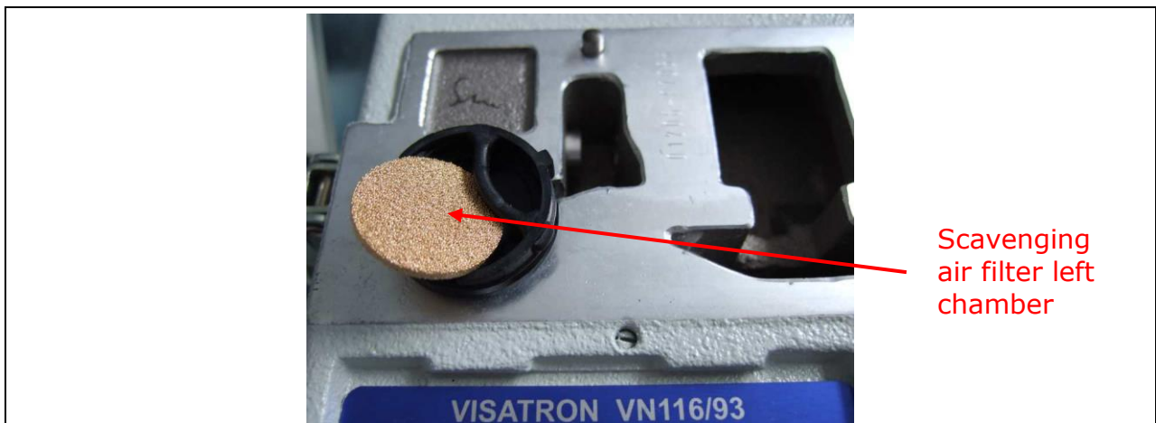
Figure 43: Exchange of the air filters
